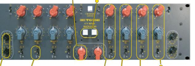
Multiply switch selects between 10 or 15db of control and changes Q, and also has a bypass select for each band.
