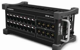
Portable rugged 16 inputs, 8 outputs stagebox with dSNAKE connection and expansion port.
