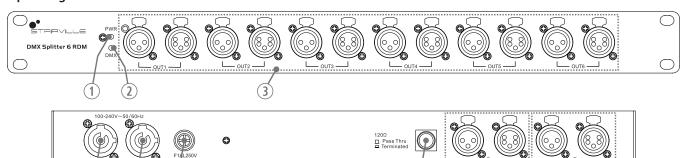
1. PWR: The red LED lights up when the device is connected to the mains.
