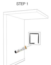
Apply Vicoustic's Flexi Glue at the back of the Multifuser DC2 acoustic panel, near the edges.
