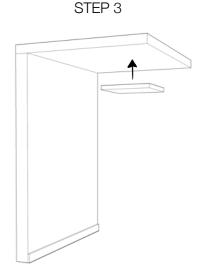
Apply the Multifuser DC2 Acoustic Panel on the ceiling surface
