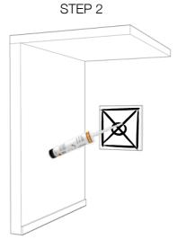
Apply Vicoustic's Flexi Glue in the centre of the Multifuser DC2 like shown on the image above.
