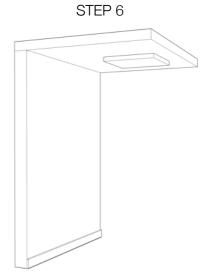
Apply again the Multifuser DC2 on the surface and hold for 2 minutes and ensure it stays fixed in place.
