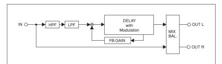
These effects modulate the delay sound. Each aspect of the sound is controlled by the following effect parameters.
