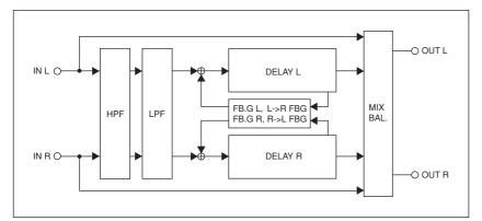
These effects add two delays; one each to the L and R channels. This is similar to Stereo Delay (page 40), but Echo mixes the L/R channel delay sounds for feedback. You can specify the amount of feedback sent from the L channel to the R channel, and from the R channel to the L channel.
