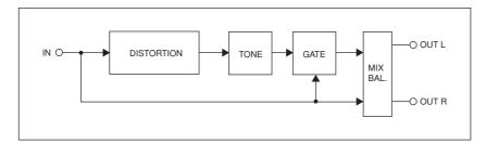
This effect distorts the sound. It is used mainly on electric guitar. Each aspect of the sound is controlled by the following effect parameters.
