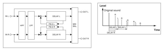
This effect adds two delayed sounds; one each for the L and R channels. You can control each delay independently. Each aspect of the sound is controlled by the following effect parameters.
