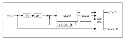
This effect adds delayed sounds to the Left, Center, and Right channels. Each delay can be controlled independently. Each aspect of the sound is controlled by the following effect parameters.
