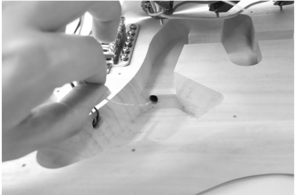
Hook the grounding cable onto the spring claw. Ensure there is sufficient contact between the stripped end of the earthing wire and the spring claw.
