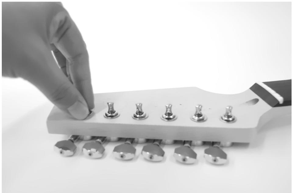
Tighten the nuts on the front with an appropriate spanner, then tighten the screws on the back firmly to fasten the tuners.
