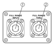
1, 2 Connections, wired in parallel (Speaker Twist)
