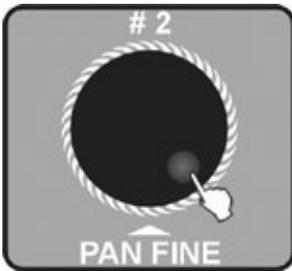
4. Use Jog wheel #2 to view the steps, the strobe display [002] indicate programmable step number.
