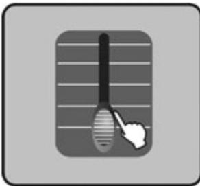
4. Move the FADERS1-24 to change COLOUR/GOBO channel values (The codes of the channel feature of ARRT CODE are "C" and "G" in the fixtures bank) output for the convenience to check other channels but the channel output will not be stored in the preset.
