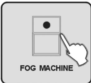
3. Control: The fog machine work as it's set in normal. Press FOG MACHINE button to output maximal fog (set 481CH output to be 255).
