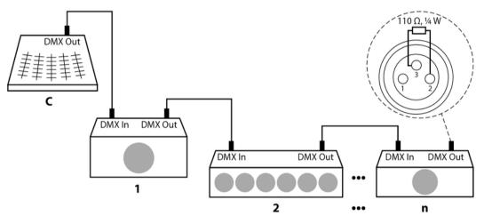
Connections in 'Master / Slave' mode When you configure a group of devices in 'Master / Slave' mode, the first unit will control the others. This feature is especially useful to start a show without much programming. Connect the DMX output of the master unit to the DMX input of the first slave unit. Then connect the DMX output of the first slave unit to the DMX input of the second slave unit and so on.
