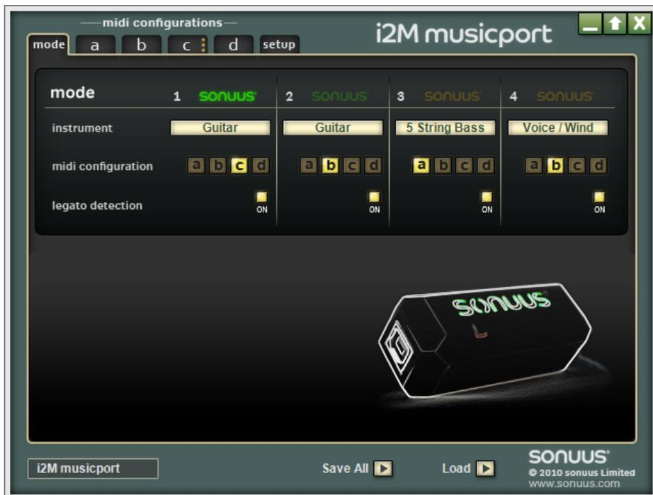
Figure 4: The **mode** tab used to edit and select Operating Modes
