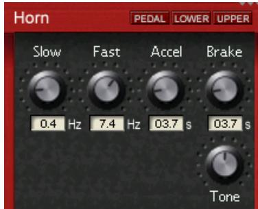
These controls are used to adjust various rotor settings. Many rotary speaker systems used a speaker for bass frequencies and a horn for treble signals, which rotated at different speeds. This rich, complex sound is faithfully reproduced and fully programmable in the B4000+.
