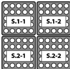
In the master-slave configuration, you can interconnect four devices of the same type to one large matrix with 10×10 LEDs. The effects then use this device combination in common.
