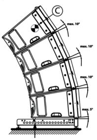
Usually, several units are so installed to a line array, that they are arranged arcuately. The figure alongside shows an example of how four elements can be combined into a system that stands on the ground (ground stack). In the figure, the centre of gravity is marked by 'C'.
