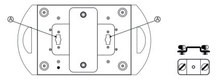
A Quick lock openings for Omega brackets
