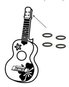
Press the four fixing rings for the machine heads from the front into the respective holes of the headstock.
