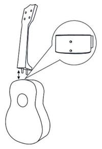
The neck is fastened with a tongue and groove connection to the body. First, check whether the connection between neck and body fits correctly. Wood slightly changes its shape over time. If the neck sits too tight in the groove on the body, a slight adjustment with a sharp wood chisel or sandpaper may be needed.
