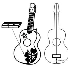
The bridge is to be glued and fixed with the two long screws on the soundboard. First mark the correct position of the bridge on the soundboard. Note the spacing dimensions shown in the figure.
