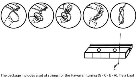
The package includes a set of strings for the Hawaiian tuning (G - C - E - A). Tie a knot at one end of the strings (simple knot for the two thicker strings, double knot for the two thinner strings) and insert the strings into the grooves of the bridge as shown in the figure:
