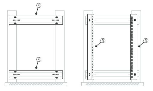
**4.** Then fix the four crossbars (4) with four Phillips-head screws M6  $\times$  15 each to the two supporting elements. Next, fix the four rack rails (5) with two cylinder head screws M6  $\times$  20 each and self-locking nuts to the two crossbars. Make sure that the rebate of the rack rails assembled points inwards as illustrated!
