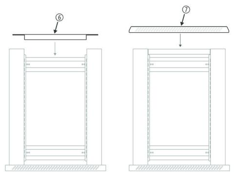
5. Place the fan base (6) between the two supporting elements. If required, you may install additional fans in this base for cooling the devices in the rack. The fan base itself is only inserted and not fixed with screws! Place the cover plate (7) of the housing on the assembled unit and fix the cover plate with four rounded head screws M8 × 20 to the two supporting elements.
