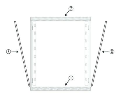
**6.** Next, insert the two side panels (8). Ensure that the two fixing pins latch properly at the lower border of each side panel in the floor plate. Tilt the side panel upwards and latch the locking mechanisms on both sides.
