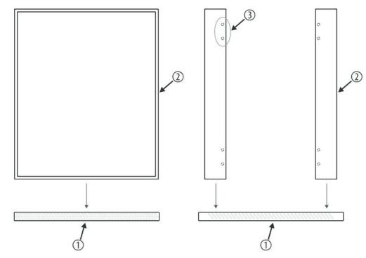
**1.** Place the two supporting elements (2) as shown in the floor plate (1). Based on the construction, the two components are fixed easily and cannot be twisted and inserted.
