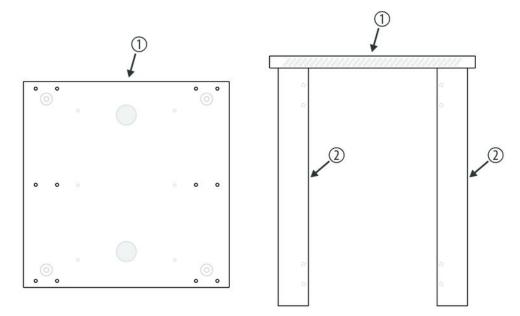
2. Turn the assembly unit in such a manner that the two supporting elements can be fixed into the floor plate with six Phillipshead screws M6 × 15 each.
