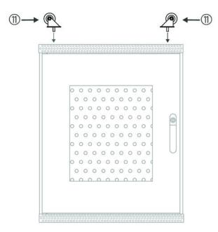
8. Place the rack with the cover plate down on a suitable assembly surface. Use a soft pad in order to avoid damaging the assembly surface or surface of the housing. Finally, assemble the four wheels (11) on the floor plate.
