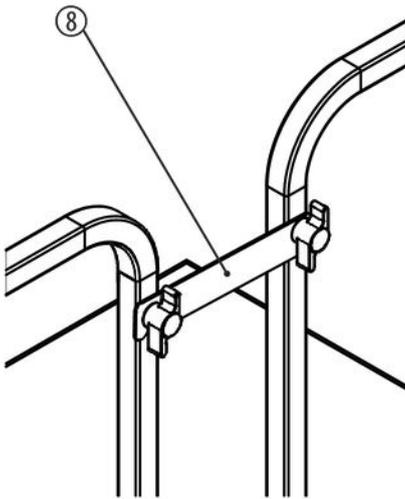
If more railings are required, attach them to the stage platforms first. Then connect the railings to each other. Either use the straight railing connectors (8) or the angled railing connectors (9). Tighten the tommy screws on the railing connectors firmly.
