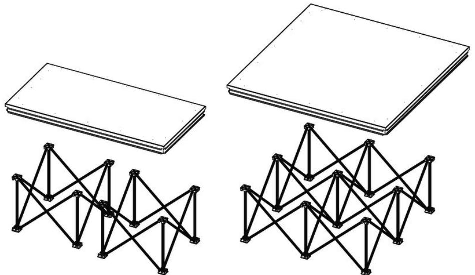
Unfold the feet completely and place them on an absolutely flat, solid and sufficiently stable ground. Put the stage platforms so on the feet, that the tops of the feet are respectively located at the corners of the stage platforms. The stage platforms must snap in on all feet.
