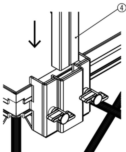
Insert the railings (4) from the top all the way into the mounting brackets.
