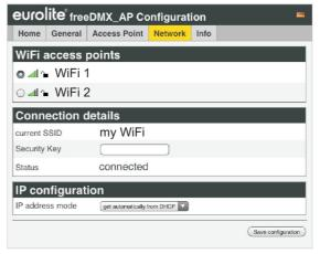
**3** Go to the "Network" tab and select the network into which you want the freeDMXAP to connect to.
