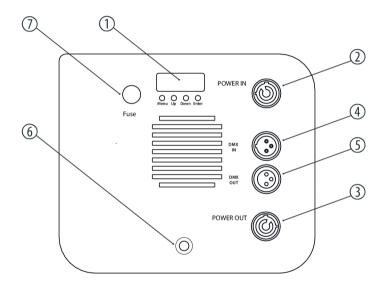
Display with function buttons. The display flashes when a valid DMX signal is present. [Enter] Confirms a selected value. [Up], [Down] Increases / decreases the displayed value by one. [Menu] Calls up the main menu or a submenu. 2 Power-Twist connector for the power supply of the device. 3 Power-Twist connector for the power supply of a further device. 4 [DMX IN] DMX input 5 [DMX OUT] DMX output
