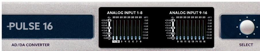
The number above the fader shows the maximum level in dBu, which the input can handle. When the fader is set to “20” like in the picture above the input can handle an maximum input level of +20dBu. Avoid exceeding this maximum level to prevent digital clipping.
