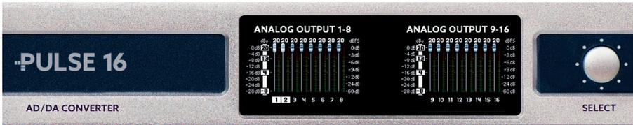
The dB scale on the right side shows the resolution of the metering levels. This scale does not show the level value of the fader!
