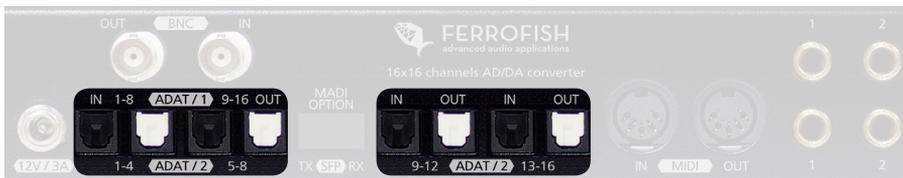
Each ADAT interface can transfer eight channels at SMUX/1. When using SMUX/2 the channel count reduces to 4. Since the PULSE16 is equipped with four ADAT interface In/ Out pairs, transfer of all analog 16 input and 16 output channels is still possible. SMUX/4 (up to 192kHz) is only enabled when the MADI MX upgrade is installed. In this case only two channels are transferred over a ADAT cable, resulting in 8 input and 8 output channels in total, using the four interface pairs.
