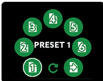
After selecting the desired preset by using the SELECT pot and MENU to load it a second screen appears. This screen lets you choose what should be loaded: The GAINS of the analog inputs, the LEVELS of the analog outputs, the routing – or all three items.
