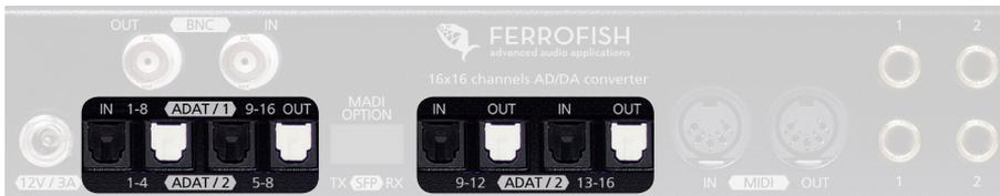
Each ADAT interface can transfer eight channels at SMUX/1. When using SMUX/2 the channel count reduces to 4. Since the PULSE16 is equipped with four ADAT interface In/ Out pairs, transfer of all analog 16 input and 16 output channels is still possible. SMUX/4 (up to 192kHz) is only enabled when the MADI MX upgrade is installed. In this case only two channels are transferred over a ADAT cable, resulting in 8 input and 8 output channels in total, using the four interface pairs.
