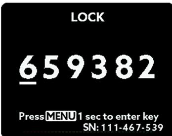
After entering the correct PIN, keep the MENU button pressed for one second. The device is locked now. Follow the same procedure to unlock the device again.
