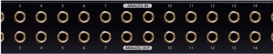
All analog inputs and output can be found on in balanced ¼" (6.3mm) TRS jacks, and can be set independently to a level/sensitivity between -8dBu and +20dBu.
