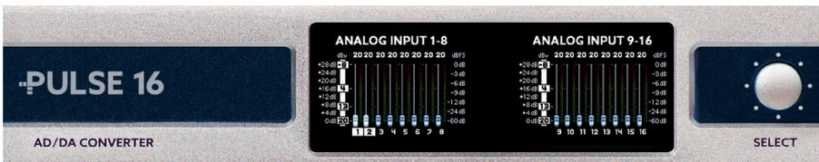
The number above the fader shows the maximum level in dBu, which the input can handle. When the fader is set to “20” like in the picture above the input can handle a maximum input level of +20dBu. Avoid exceeding this maximum level to prevent digital clipping.
