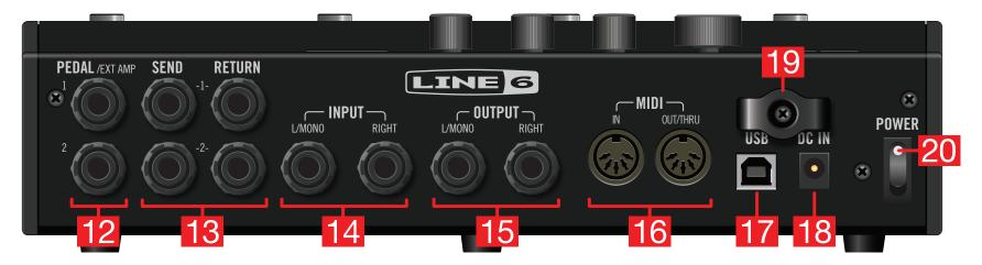
**12. PEDAL/EXT AMP 1-2** Two expression pedals can be connected to the HX Effects device and assigned to adjust a wide variety of parameters. By default, EXP 1 is automatically assigned to control and bypass Wah/Pitch Wham type blocks, and EXP 2 is automatically assigned to control Volume blocks, making them ready for use with your connected expression pedal(s). See "Assigning a Controller"
