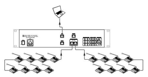
Up to 16 call stations can be connected in 2 lines to the control centre.
