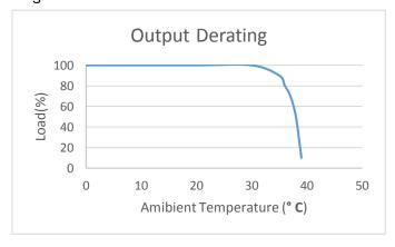
When internal temperature is higher than the limit, the thermal control system will gradually lower the intensity of the connected strips or dots to cool down the driver. Once the internal temperature is within the limit, the driver will resume its normal operation.
