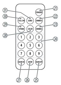
To use the remote control, point its infrared diode at the infrared sensor on the unit and press the desired buttons. The maximum operating distance is about 9 m. The device will only respond to the remote control signals if it is not controlled via DMX.
