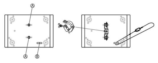
The threads on the bottom side of the housing (A) allow the secure attachment of the included mounting bracket. There, you can fasten adapters such as half couplers, trigger clamps, c-hooks etc. Safety cables are being threaded through the eyelet (B) on the bottom side of the housing.
