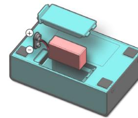
\* Make sure the "+" and "-" ends of the battery are oriented correctly.
