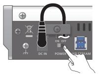
3. Turn on the power in the order of source devices → output devices.
