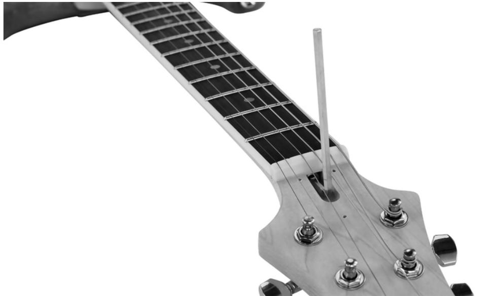
Screw the cover for the truss bar onto the header headstock.
