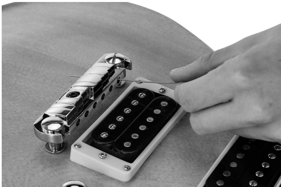
Tighten the strings around the tailpiece as shown and thread the strings into the holes in the tuners. Wrap the end of the string a few times around the peg and first hand-tighten each string. Make sure that the individual strings are in the correct nut position.
