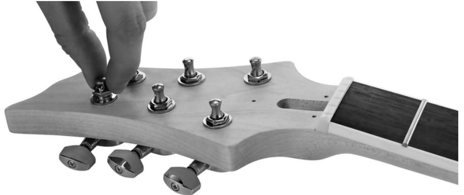
Tighten the nuts on the front with an appropriate spanner, then tighten the screws on the back firmly to fasten the tuners.
