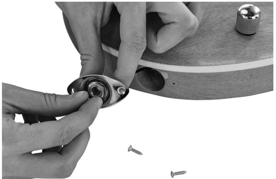
Then screw the holder of the output socket to the body with the screws provided.
