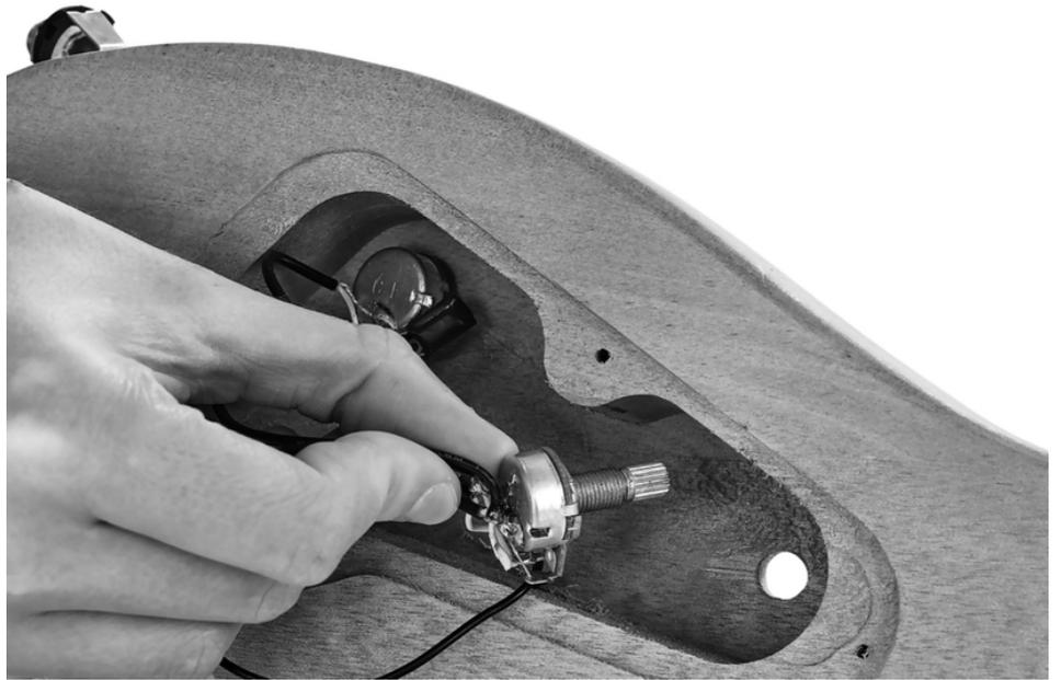
Turn the guitar over and fix the pots and switch with the supplied washers and nuts on the front of the body.
