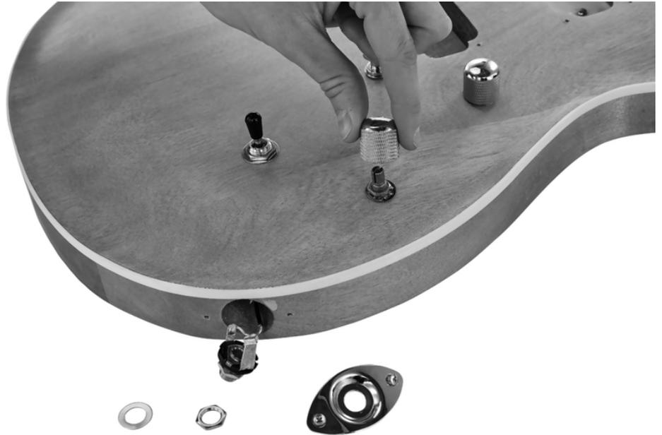
Insert the holder for the output socket and check the projection of the socket. This must protrude so far over the bracket to the outside that it can be sufficiently tightened with the supplied nut and then only slightly protrudes. If necessary, correct the protrusion by turning the counter nut inside accordingly.
