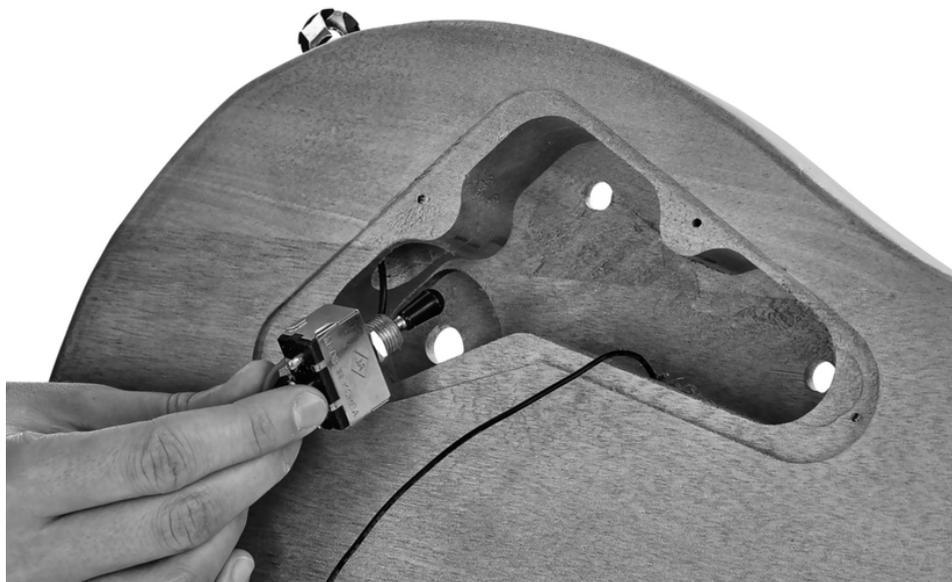
Insert the pots into the back slots as shown in the following illustrations.
