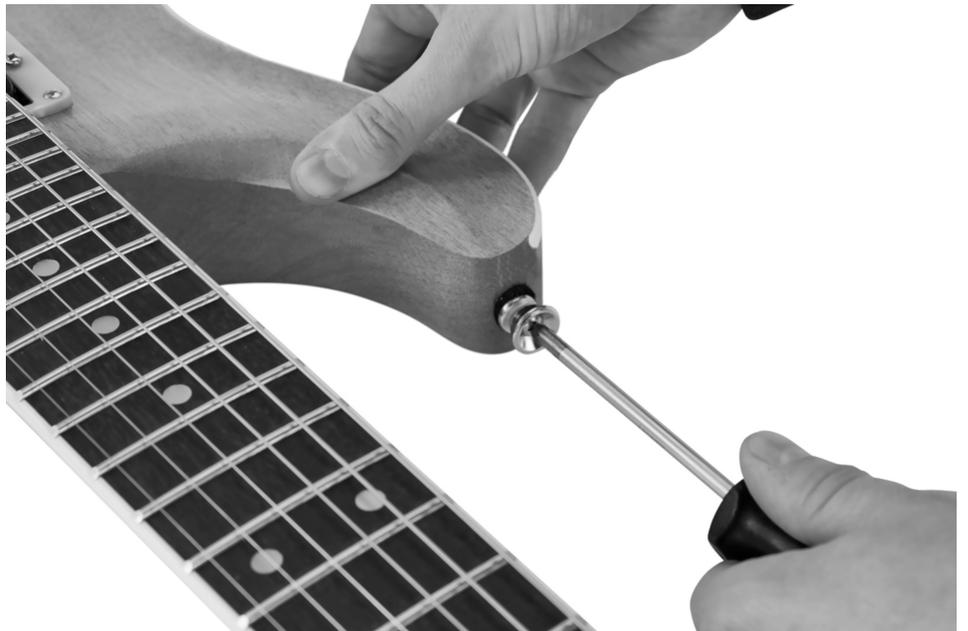
Slide the tailpiece onto the mounting bolts as shown. The tailpiece is still loose and is only fixed when stringing the guitar.
