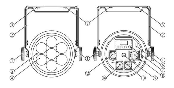
1 Locking screws for the brackets. 2 Two-piece bracket for hanging or floor setup 3 Omega bracket with quick lock 4 LED 5 Infrared sensor for optional remote control 6 Safety cable eyelet. 7 Display and keypad [MODE] Activates the main menu, toggles between the menu levels or closes a submenu. [DOWN] Decreases the displayed value by one. [UP] Increases the displayed value by one.
