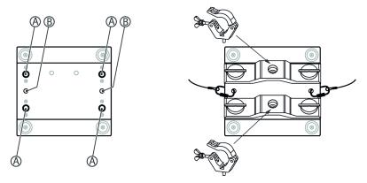
The Quick Lock mounts on the bottom side of the housing (A) allow the secure attachment of the included mounting brackets. There, you can fasten adapters such as half couplers, trigger clamps, c-hooks etc. Safety cables are being threaded through the safety eyelets (B) on the bottom side of the housing.
