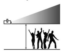
In order to meet the limits for maximum irradiation (MZB limit value for the non-hazardous irradiation of the eye or the skin with a laser), the device must be installed at a height of at least 2.7 m according to the BGV-B2 valid in Germany.
