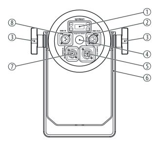
Display and keypad [MENU] Activates the main menu, toggles between the menu levels or closes a submenu. [DOWN] Decreases the displayed value by one. [UP] Increases the displayed value by one. [ENTER] Opens a submenu or confirms a value. 2 [DMX OUT] DMX output, designed as 3-pin XLR panel socket (IP65) 3 Locking screws for the brackets. 4 Pressure compensation element
