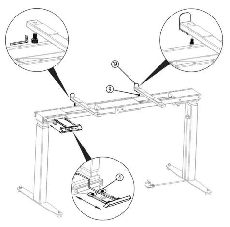
12. Attach the angle pieces (19) if desired with one Allen screw M6×10 each (9) to the crossbars (16).
