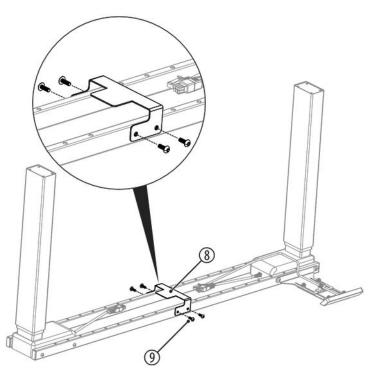
**5.** Attach the motor holder (8) with four Allen screws M6×10 (9) to both tubes (6) using the Allen key (20).
