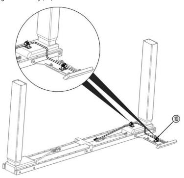
**6.** Attach two adhesive cable ties (10) in the illustrated position to properly install the cable of the control panel.
