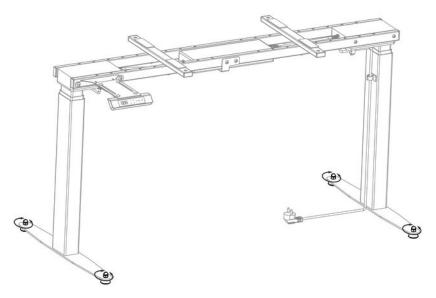
**13.** Align the adjustable feet to compensate for the floor unevenness.
