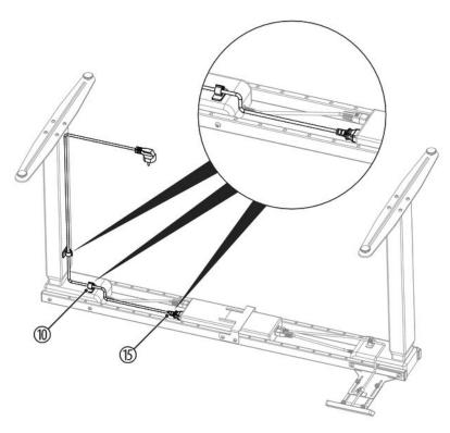
**9.** Attach two adhesive cable ties (10) in the illustrated position to properly install the power cable (15). Connect the power cable (15) to the motor (11).
