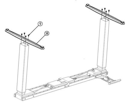
8. Attach the feet (14) with four Allen screws M6×10 each (9) to the standing columns (7).
