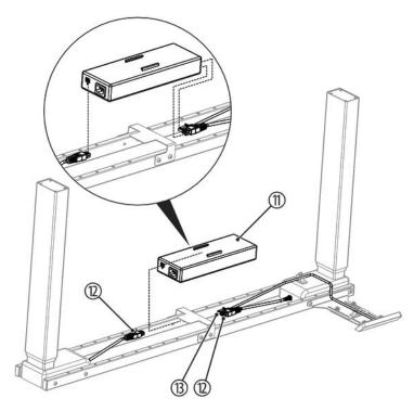
Slide the motor (11) in the holder (8) and connect the cables of the standing columns (12) and the cable of the control panel (13) to the motor.
