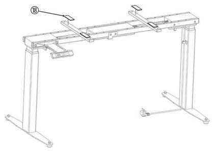
11. Attach two adhesive foam pads (18) to each crossbar (16) at the desired positions.
