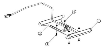
**3.** First attach the control panel (1) to the control panel holder (2). Use the four supplied slide screws (3) and the four round nuts (4) and hand-tighten them.
