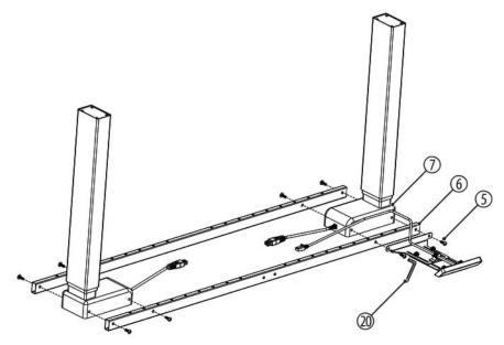
**4.** Place the tubes (6) and standing columns (7) as illustrated. Attach the mounted control panel holder with two Allen screws M6×25 (5) to the tube (6) and to the standing column (7) using the Allen key (20). Attach the tube and the standing column on the other side following the same procedure.
