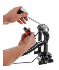
Step 2: Snap the pedal bracket into the frame of the pedal
