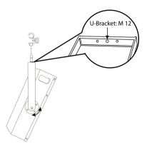
The optionally available vertical and horizontal mounting brackets (U brackets) allow you to attach the speaker stably and securely to the wall, ceiling or half coupler and thus to trusses.
