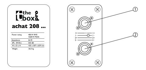
1, 2 NL4 connections wired in parallel (1+,1- through-connected and assigned; 2+, 2- through-connected and not assigned)
