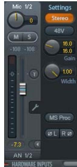
**Width.** Setting the stereo width. 1.00 equals full stereo, 0.00 mono, -1.00 swapped channels.
