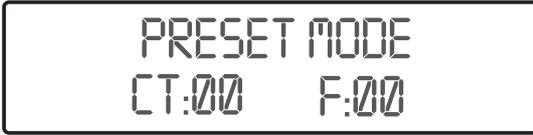
Press the ENTER button to select flash speed, respectively. You can select the desired values via the UP or DOWN buttons.
