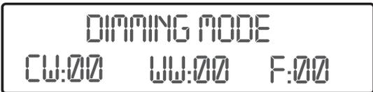
Press the ENTER button to select the brightness of the cold white and the warm white LEDs and the flash speed, respectively. You can select the desired values via the UP or DOWN buttons.
