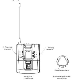
Transmitter charging contact locations are as shown. A bodypack transmitter contains three contacts; one on the left side, and two on the right side. These must align with the single and dual contacts of the charger slot. The handheld transmitter contains three charging contacts located toward the tail end of the transmitter; one on the left side, and two on the right as shown. These must align with the single and dual contacts of the charger slot.
