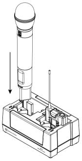
Only one transmitter may be seated into either side at a time; one bodypack, or one handheld, but not both together.
