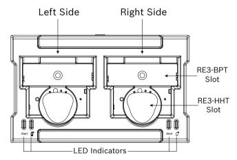
The BC2 contains two sides as shown; left and right. Each side contains a bodypack transmitter slot and a handheld transmitter slot. When properly seated into a slot, the transmitter's charging contacts will be in contact with the charger's pins.
