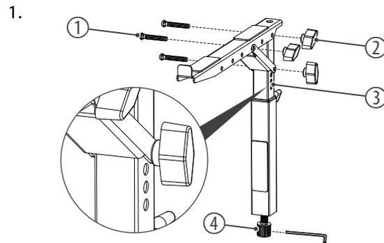
Attach the support brackets with the screws (1) and the locking screws (2) to the tube (3).
