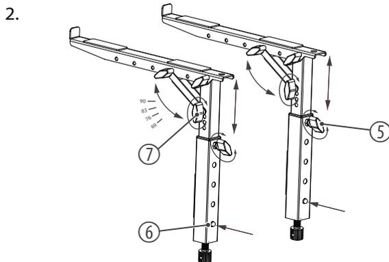
Loosen the locking screw (5) for adjusting the height of the support brackets. Press the safety bolt (6) at the tube and pull the support brackets simultaneously upwards until the safety bolt snaps in at the desired height. Tighten the locking screw (5).
