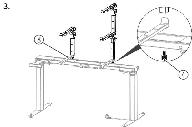
Attach the extensions to the crossbars (8) of the Multi Electric Stand (item no. 491963, separately available) with one 3/8" cylinder head screw (4) each using the Allen key.
