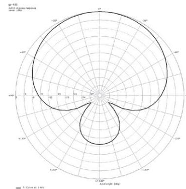
Polardiagramm @ 1 kHz
