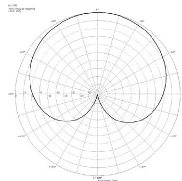
Polardiagramm @ 1 kHz
