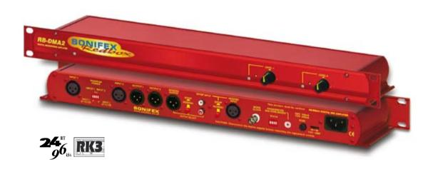
// The unit can either be used as two independent microphone amplifiers, or one mic input can be copied to both channels of the digital output. //
