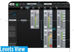
In the Levels View, you can set input and output levels for each channel and set limiter response. Buttons on each fader block provide quick access to mute, EQ and delay for each channel as well as polarity reversal ("Phase Inverted"). Levels view will differ depending on selection of stereo or 2-way mode.
