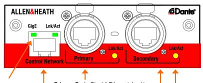
Link status One LED indicates network activity. The other indicates that a Gigabit Ethernet link has been established.
