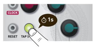
Unplug all CV inputs and **hold the TAP (reset) button** for a second to adjust Grids' settings. Refer to the **diagram on the next pages** for a list of all available settings. The 3 LEDs indicate the value of the setting being modified. Hold the TAP (reset) button again for a second when you are done.
