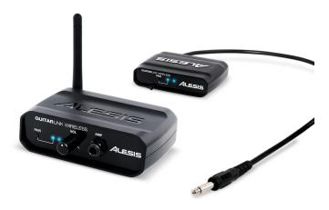
The GuitarLink Wireless is an instrument wireless system that occupies the 2.4 GHz digital wireless spectrum.
