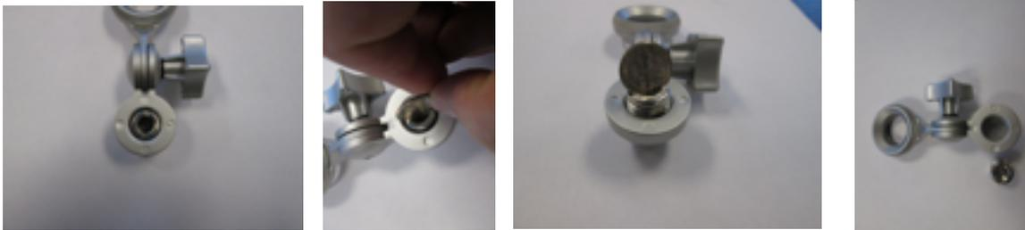
**European stand connector from the bottom of the swivel mount.The most effective method is to use a coin,lock it into the adapter and twist the coin clockwise. The adapter should start to detach after about 3-5 rotations of the coin.**
