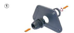
1. Assemble strain relief into the end piece with the hole.
