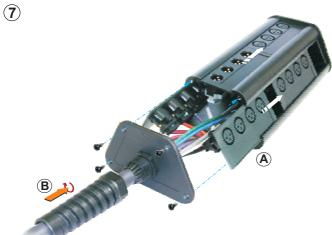
7. (A) Slide in the assembled connector plates into the extensions and screw on the end piece with 4 screws.
