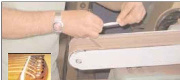
Proper saddle fit and break angle
