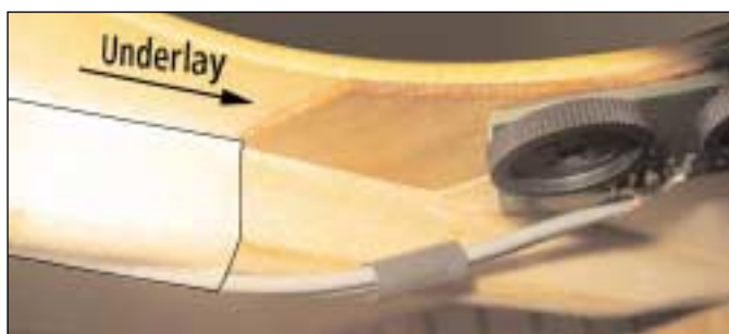
Paper masking tape as strain relief, underlay and Sound Hole Control
